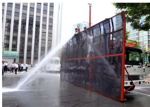
Pic. 11 - The vehicle "transformed" into a wall.
